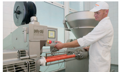
Revolver head for reduced casing change times
